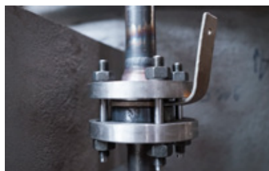
Adjustment orifice plate for regulation of the amount of steam for the injection
