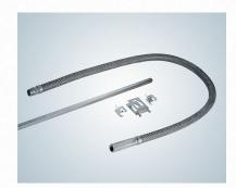
The construction of the hose allows a flexible positioning of the sprinkler head. Compared to the usual assembly technology, this results in considerable time and cost savings. The supplied mounting brackets allow mounting to the substructures of all common ceiling systems.
